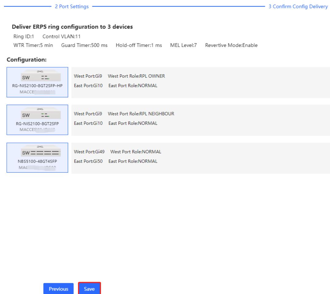
After all cables are connected according to the topology, the devices will automatically form an ERPS ring.
