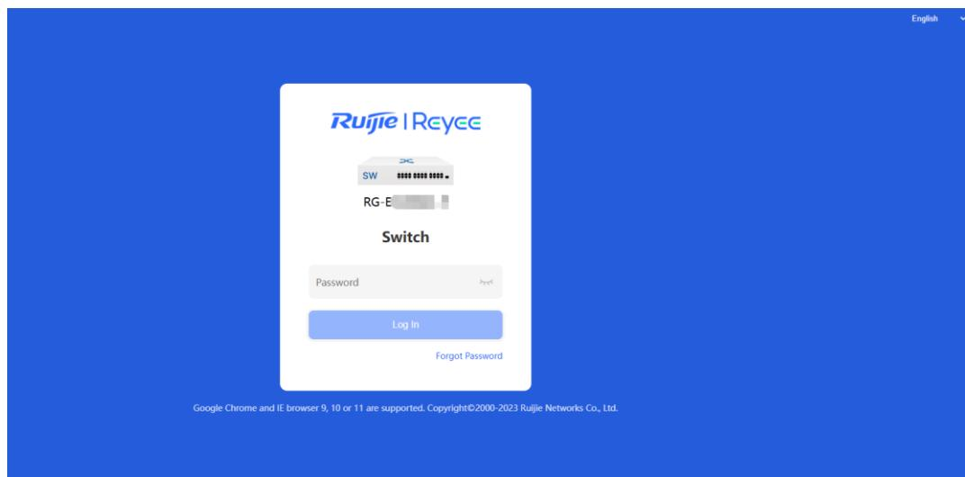
If you forget the device's IP address or password, hold down the **Reset** button on the device panel for more than 5 seconds to restore factory settings when the device is connected to the power supply. After restoration, you can use the default IP address to log in to the device and then change the login password.
