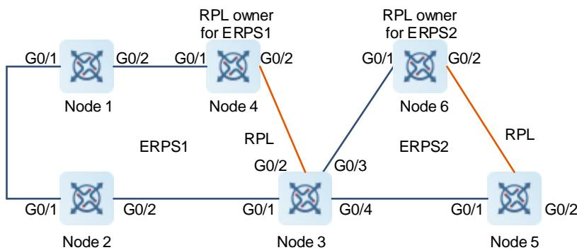
As shown in [Figure 1-24](#), the link between node 3 and node 4 is the RPL of the Ethernet ring ERPS 1. As the RPL owner node of ERPS 1, node 4 blocks the RPL port. The link between node 5 and node 6 is the RPL of the Ethernet ring ERPS 2. As the RPL owner node of ERPS 2, node 6 blocks the RPL port. ERPS 1 (node 1-2-3-4) and ERPS 2 (node 3-5-6) share node 3, forming a tangent-ring topology. Node 3 is the tangent node.
